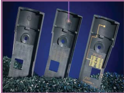
Laser activation. (Image Courtesy of LPKF Laser & Electronics.)
