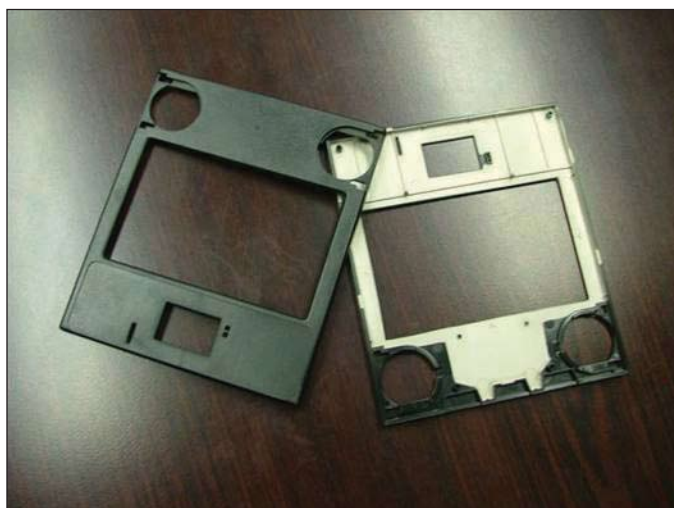
Figure 1: Selectively copper and nickel-plated enclosures for EMI shielding
