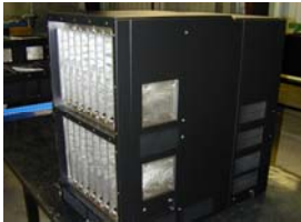
Plated Plastic Router Chassis
